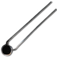
143 Series, 2,54 mm [0.1 in] disc thermistor with leads and epoxy, 3,000 Ohm resistance, \pm 10.0\% tolerance, 25/85 BETA = 3974
