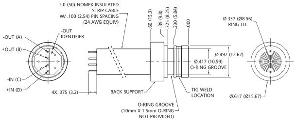
**Note:** Non-concentricity effects at the diaphragm weld area may cause runout of up to ±0.006" between the upper and lower portions of the sensor body. (It is recommended to use a counter bore to mate with this device to allow for this non-concentricity.)
