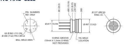
Note: Non-concentricity effects at the diaphragm weld area may cause runout of up to  $\pm 0.006$ " between the upper and lower portions of the sensor body. (It is recommended to use a counter bore to mate with this device to allow for this non-concentricity.)
