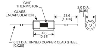
Thermistors change resistance with a change in temperature. They do not amplify, rectify, polarize or generate a signal. The thermistor temperature may be changed by the surrounding temperature or by self-heating the thermistor by passing a current through it.
