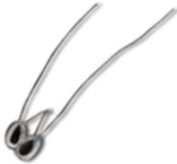
126 Series, matched large glass bead, 100,000 Ohm resistance, \pm 1,0\text{ }^{\circ}\text{C} [1.8 ^{\circ}\text{F} ] tolerance, 25/85 BETA = 3669
