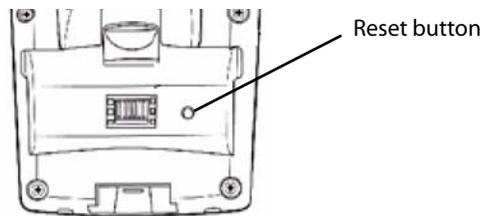
*This shows the back of the computer inside the battery compartment.*
