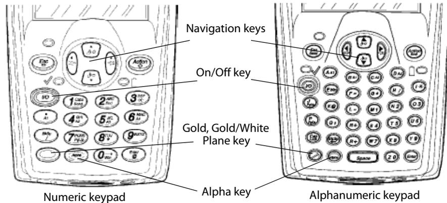
Use the following sections to understand how to use the keypad. For information on remapping the keypad, you can download the Device IDL Resource Kit from the Intermec web site at [www.intermec.com/idl](http://www.intermec.com/idl).
