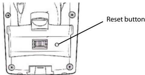
*This illustration shows the back of the computer inside the battery compartment.*
