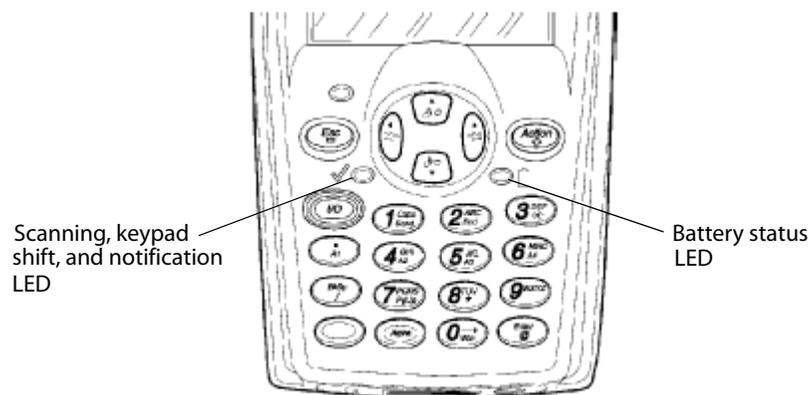
The battery status LED (B) and the scanning/keypad shift and notification LED (C) turn red, green, or yellow to indicate the status of the battery, scanner information, and the mode of the keypad.
