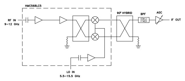
Note: LSB and USB is determined by GND on Hybrid
