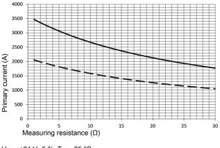
$\label{eq:UC} \begin{array}{l} ---- U_C = \pm 24 \; V \; -5 \; \%, \; T_A = 85 \; ^\circ C \\ ---- U_C = \pm 15 \; V \; -5 \; \%, \; T_A = 85 \; ^\circ C \\ \\ \mbox{Primary currents higher than } I_{PM} \; \mbox{only for peak!} \end{array}$
