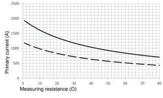
$\label{eq:UC} \begin{array}{l} ---- U_C = \pm 24 \; V \; -5 \; \%, \; T_A = 85 \; ^\circ C \\ ---- U_C = \pm 15 \; V \; -5 \; \%, \; T_A = 85 \; ^\circ C \\ \\ \mbox{Primary currents higher than } I_{PM} \; \mbox{only for peak!} \end{array}$
