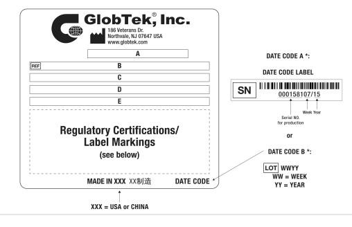
A=USB Adaptive Power Source ICT/ITE/Medical Power supply B=P/N: (料号) WR9QZ900USBPPSCIMR6B C=Model (型号) GTM96181-18PD-PPS D=Input (输入)100-240V~, 50-60 Hz, 1.2A
