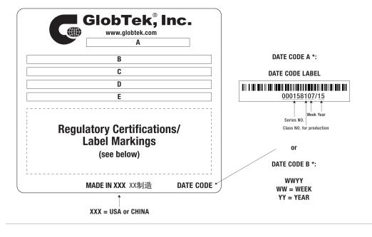
A=ICT/ITE Power Supply B=P/N: (料号) WR9QZ900LCP-N(R6B) C=Model (型号) GT-46180-1824-4.0 D=Input (输入)100-240V~, 50-60 Hz, 0.6 A E=Output (输出)20.0 V === 0.9 A, 18.00W
