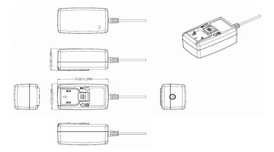
LED INDICATOR: Green Power ON indicator LED standard. May be ordered without LED as an option, for cost reduction.
