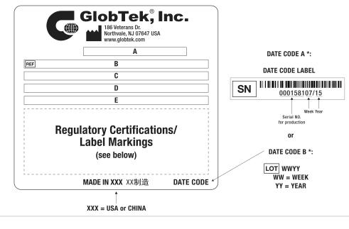
A=Medical/ICT/ITE/Household use Power Supply B=P/N: (料号) WR9QX833LCPNNAR6B C=Model (型号) GTM46402-4048 D=Input (输入)100-240V~, 50-60 Hz, 1.0A E=Output (输出)48.0 V === 0.83 A, 40.00W
