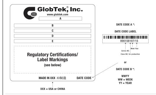
A=ICT / ITE / Medical Power Supply/Class 2/Household Power Supply B=P/N: (料号) WR9QR200T00NAIMR6B C=Model (型号) GTM96060-0636-6.0 D=Input (输入)100-240V~, 50-60 Hz, 0.6 A E=Output (输出)30.0 V == 0.2 A, 6.00W
