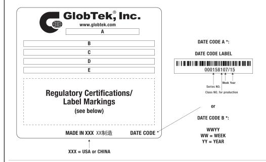
A=ICT / ITE / Medical Power Supply/Class 2/Household Power Supply B=P/N: (料号) WR9QI750T00NAIMR6B C=Model (型号) GTM96180-1830-6.0 D=Input (输入)100-240V~, 50-60 Hz, 0.6 A E=Output (输出)24.0 V == 0.75 A, 18.00W
