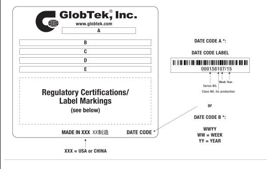
A=ICT/ITE Power Supply B=P/N: (料号) WR9QI500CCPNA-N(R6B C=Model (型号) GT-46120-1224 D=Input (输入)100-240V~, 50-60 Hz, 0.6A E=Output (输出)24.0 V === 0.5 A, 12.00W
