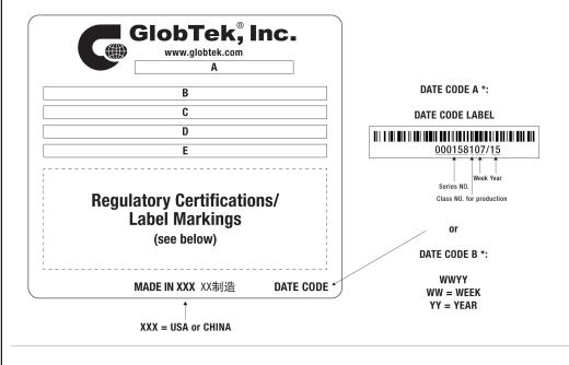
A=ICT/ITE Power Supply B=P/N: (料号) WR9QI250LCPNA-N(R6B) C=Model (型号) GT-46060-0624 D=Input (输入)100-240V~, 50-60 Hz, 0.3 A E=Output (输出)24.0 V === 0.25 A, 6.00W
