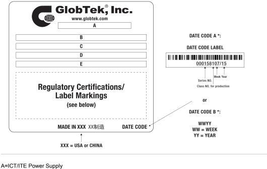
B=P/N: (料号) WR9QI250LCP-N(R6B) C=Model (型号) GT-46060-0624 D=Input (输入)100-240V~, 50-60 Hz, 0.3 A E=Output (输出)24.0 V === 0.25 A, 6.00W
