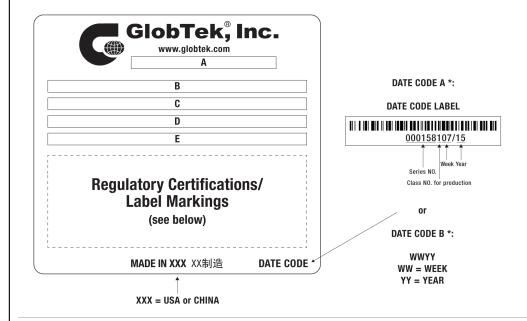
A=ICT / ITE / Medical Power Supply/Class 2/Household Power Supply B=P/N: (料号) WR9Ql250LCP-IMR6B C=Model (型号) GTM96060-0624 D=Input (输入)100-240V~, 50-60 Hz, 0.6 A E=Output (输出)24.0 V === 0.25 A, 6.00W
