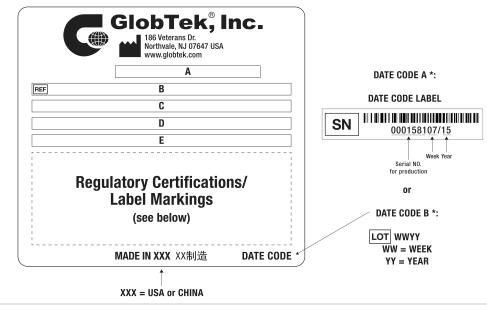
A=Medical/ICT/ITE/Household use Power Supply B=P/N: (料号) WR9QI1660LCPN(R6B) C=Model (型号) GTM46402-4024 D=Input (输入)100-240V~, 50-60 Hz, 1.0A E=Output (输出)24.0 V === 1.66 A, 40.00W
