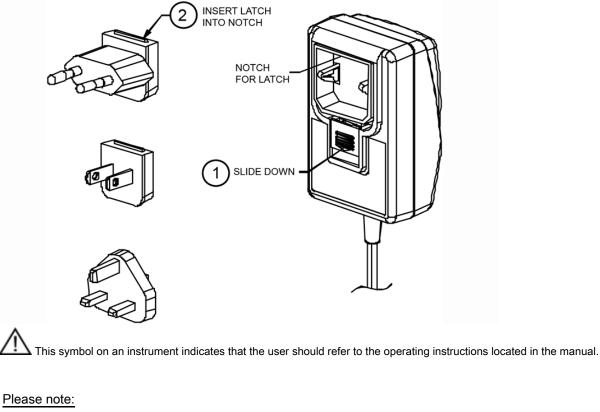
The blades shown above are for representation of the installation process and do not indicate which AC blades are included with this power supply. Please reference the specifications "Power Supply Information" (page 2) and "Input Configuration (page 6) for information regarding the actual blade included with this power supply, if any.
