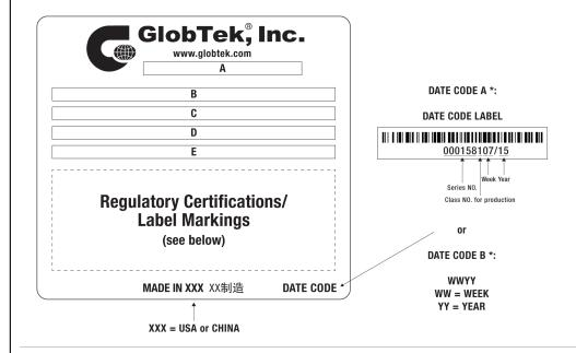
A=ICT / ITE / Medical Power Supply/Class 2/Household Power Supply B=P/N: (料号) WR9QH333T00NAIMR6B C=Model (型号) GTM96060-0618 D=Input (输入)100-240V~, 50-60 Hz, 0.6 A E=Output (输出)18.0 V === 0.33 A, 6.00W
