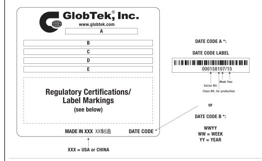
A=ICT / ITE / Medical Power Supply/Class 2/Household Power Supply B=P/N: (料号) WR9QG400T00NAIMR6B C=Model (型号) GTM96060-0615 D=Input (输入)100-240V~, 50-60 Hz, 0.6 A E=Output (输出)15.0 V == 0.4 A, 6.00W
