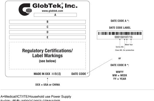
B=P/N: (料号) WR9QG2667LCPNNAR6B C=Model (型号) GTM46402-4015 D=Input (输入)100-240V~, 50-60 Hz, 1.0A
