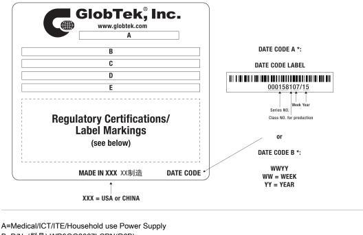
B=P/N: (料号) WR9QG2667LCPN(R6B) C=Model (型号) GTM46402-4015 D=Input (输入)100-240V~, 50-60 Hz, 1.0A E=Output (输出)15.0 V == 2.66 A, 40.00W
