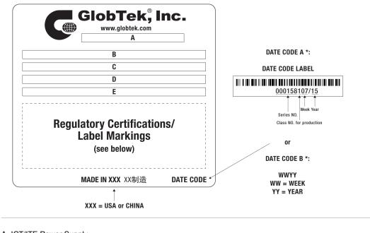
A=ICT/ITE Power Supply B=P/N: (料号) WR9QG1200LCP-N(R6B) C=Model (型号) GT-46180-1815 D=Input (输入)100-240V~, 50-60 Hz, 0.6 A E=Output (输出)15.0 V === 1.2 A, 18.00W
