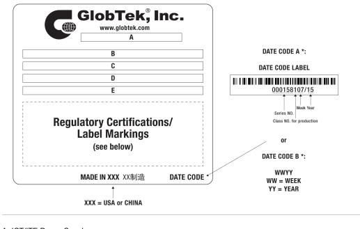
A=ICT/ITE Power Supply B=P/N: (料号) WR9QG1000CCP-N(R) C=Model (型号) GT-41052-1515 D=Input (输入)100-240V~, 50-60 Hz, 0.6 A E=Output (输出)15.0 V === 1.0 A, 15.00W
