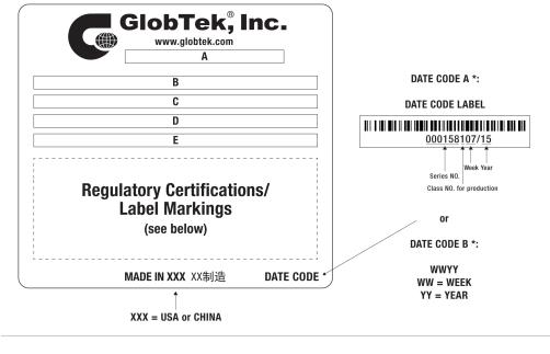
A=Medical/ICT/ITE/Household use Power Supply B=P/N: (料号) WR9QF550T00CIMCCR6B C=Model (型号) GTM96060CC0612-1.0 D=Input (输入)100-240V~, 50-60 Hz, 0.6 A E=Output (输出)11.0 V === 0.54 A, 6.00W
