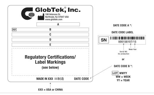
A=Medical/ICT/ITE/Household use Power Supply B=P/N: (料号) WR9QF550LCPCIMCCR6B C=Model (型号) GTM96060CC0612-1.0 D=Input (输入)100-240V~, 50-60 Hz, 0.6 A E=Output (输出)11.0 V == 0.54 A, 6.00W
