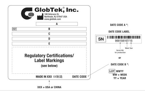
A=ICT / ITE / Medical Power Supply/Class 2/Household Power Supply B=P/N: (料号) WR9QE917CCPCK2TR6B C=Model (型号) GTM96180-1117.9-5.9 D=Input (输入)100-240V~, 50-60 Hz, 0.6 A E=Output (输出)12.0 V === 0.91 A, 11.00W
