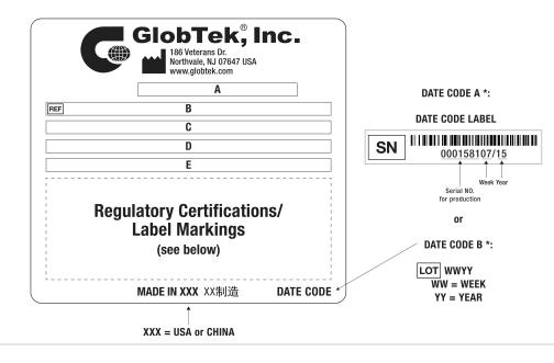
A=ICT / ITE / Medical Power Supply/Class 2/Household Power Supply B=P/N: (料号) WR9QE500T00NAIMR6B C=Model (型号) GTM96060-0612 D=Input (输入)100-240V~, 50-60 Hz, 0.6 A E=Output (输出)12.0 V === 0.5 A, 6.00W
