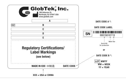
A=ICT / ITE / Medical Power Supply/Class 2/Household Power Supply B=P/N: (料号) WR9QE500LCPNAIMR6B C=Model (型号) GTM96060-0612 D=Input (输入)100-240V~, 50-60 Hz, 0.6 A E=Output (输出)12.0 V === 0.5 A, 6.00W
