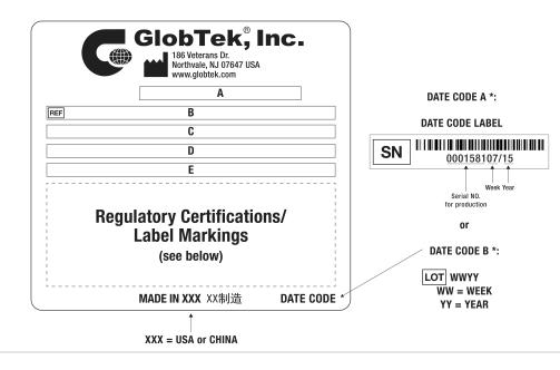
A=ICT / ITE / Medical Power Supply/Class 2/Household Power Supply B=P/N: (料号) WR9QE500CCPNAIMR6B C=Model (型号) GTM96060-0612 D=Input (输入)100-240V~, 50-60 Hz, 0.6 A E=Output (输出)12.0 V === 0.5 A, 6.00W
