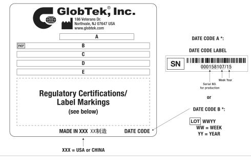
A=Medical/ICT/ITE/Household use Power Supply B=P/N: (料号) WR9QE3000LRPCIM(R6B) C=Model (型号) GTM46402-3612 D=Input (输入)100-240V~, 50-60 Hz, 1.0A E=Output (输出)12.0 V === 3.0 A, 36.00W
