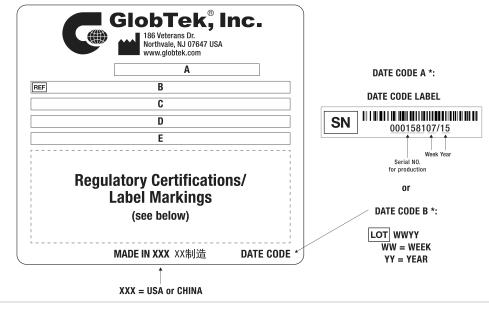
A=Medical/ICT/ITE/Household use Power Supply B=P/N: (料号) WR9QE3000LCPNNAR6B C=Model (型号) GTM46402-3612 D=Input (输入)100-240V~, 50-60 Hz, 1.0A E=Output (输出)12.0 V === 3.0 A, 36.00W
