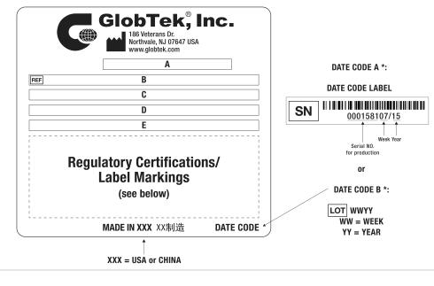
A=Medical/ICT/ITE/Household use Power Supply B=P/N: (料号) WR9QE3000LCPN(R6B) C=Model (型号) GTM46402-3612 D=Input (输入)100-240V~, 50-60 Hz, 1.0A E=Output (输出)12.0 V === 3.0 A, 36.00W
