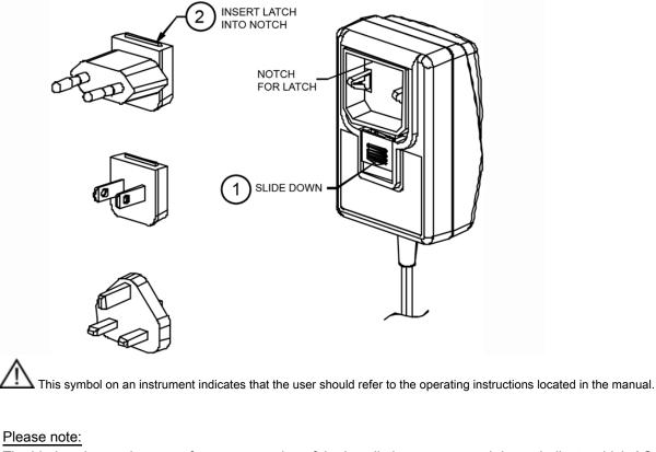
The blades shown above are for representation of the installation process and do not indicate which AC blades are included with this power supply. Please reference the specifications "Power Supply Information" (page 2) and "Input Configuration (page 6) for information regarding the actual blade included with this power supply, if any.
