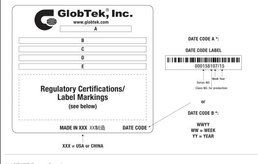
A=ICT/ITE Power Supply B=P/N: (料号) WR9QE1500LCPNNAR6B C=Model (型号) GT-46180-1812 D=Input (输入)100-240V~, 50-60 Hz, 0.6 A E=Output (输出)12.0 V === 1.5 A, 18.00W
