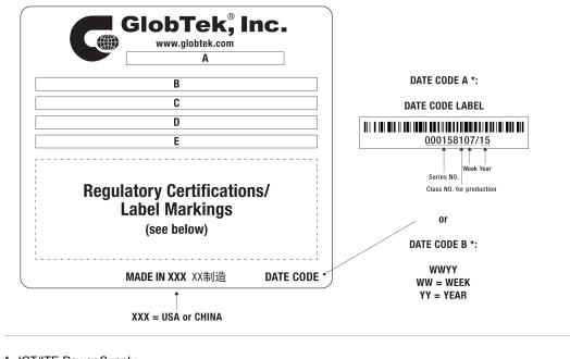
A=ICT/ITE Power Supply B=P/N: (料号) WR9QE1500CCP-N(R6B) C=Model (型号) GT-46180-1812 D=Input (输入)100-240V~, 50-60 Hz, 0.6 A E=Output (输出)12.0 V === 1.5 A, 18.00W
