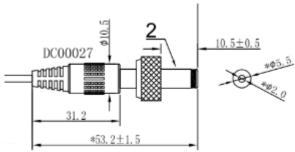
1. CRITICAL FOR LOCKING NUT TO BE FULLY THREADED.2. THREAD INSPECTION OF LOCKING NUT BEFORE SHIPPING FROM PRODUCTION IS REQUIRED.
