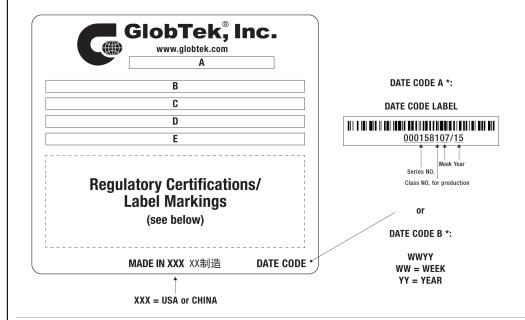
A=ICT / ITE / Medical Power Supply/Class 2/Household Power Supply B=P/N: (料号) WR9QE1250T00NACFR6B C=Model (型号) GTM96180-1517.9-5.9-CF D=Input (输入)100-240V~, 50-60 Hz, 0.6 A E=Output (输出)12.0 V === 1.25 A, 15.00W
