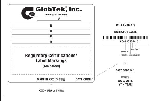
A=ICT/ITE Power Supply B=P/N: (料号) WR9QE1000LCPNA-N(R6B C=Model (型号) GT-46120-1212 D=Input (输入)100-240V~, 50-60 Hz, 0.6A E=Output (输出)12.0 V === 1.0 A, 12.00W
