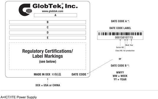
B=P/N: (料号) WR9QD660LCP-N(R6B) C=Model (型号) GT-46060-0609 D=Input (输入)100-240V~, 50-60 Hz, 0.3 A E=Output (输出)9.0 V == 0.66 A, 6.00W
