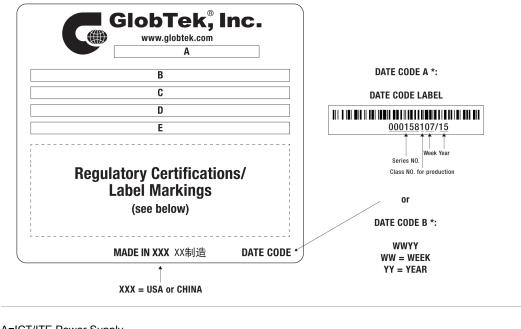
A=ICT/ITE Power Supply B=P/N: (料号) WR9QD2000LCP-N(R6B) C=Model (型号) GT-46180-1809 D=Input (输入)100-240V~, 50-60 Hz, 0.6 A E=Output (输出)9.0 V == 2.0 A, 18.00W
