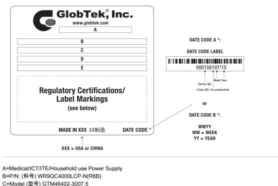
D=Input (输入)100-240V~, 50-60 Hz, 1.0A E=Output (输出)7.5 V === 4.0 A, 30.00W
