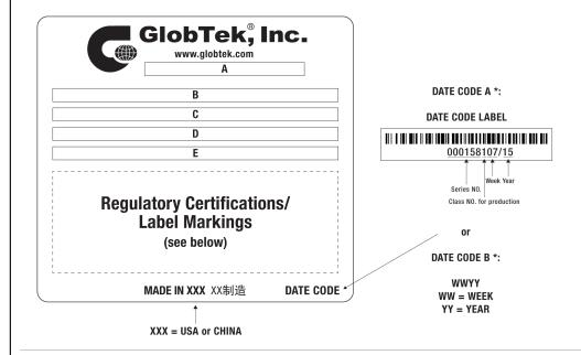
A=ICT / ITE / Medical Power Supply/Class 2/Household Power Supply B=P/N: (料号) WR9QC2400T00NAIMR6B C=Model (型号) GTM96180-1811-3.5 D=Input (输入)100-240V~, 50-60 Hz, 0.6 A E=Output (输出)7.5 V == 2.4 A, 18.00W
