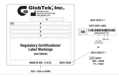
A=ICT / ITE / Medical Power Supply/Class 2/Household Power Supply B=P/N: (料号) WR9QB1000LCPCIMR6B C=Model (型号) GTM96060-0606-0.05 D=Input (输入)100-240V~, 50-60 Hz, 0.6 A E=Output (输出)5.95 V === 1.0 A, 6.00W
