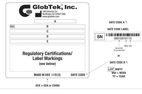
A=Medical/ICT/ITE/Household use Power Supply B=P/N: (料号) WR9QA6000LCP-N(R6B) C=Model (型号) GTM46402-3005 D=Input (输入)100-240V~, 50-60 Hz, 1.0A E=Output (输出)5.0 V == 6.0 A, 30.00W
