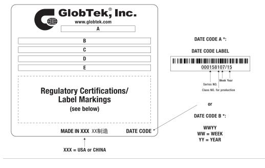
A=ICT/ITE Power Supply B=P/N: (料号) WR9QA3200K9PNNAR6B C=Model (型号) GT-46180-1605 D=Input (输入)100-240V~, 50-60 Hz, 0.6 A E=Output (输出)5.0 V == 3.2 A, 16.00W
