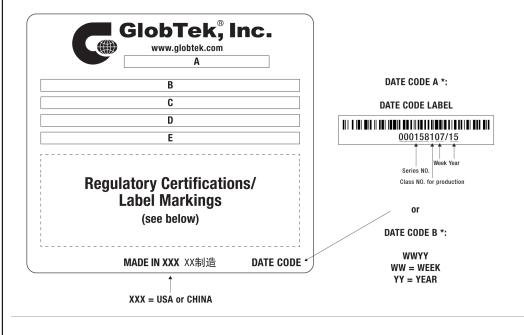
A=ICT/ITE Power Supply B=P/N: (料号) WR9QA3200CCPNA-N(R6B C=Model (型号) GT-46180-1605 D=Input (输入)100-240V~, 50-60 Hz, 0.6 A E=Output (输出)5.0 V == 3.2 A, 16.00W
