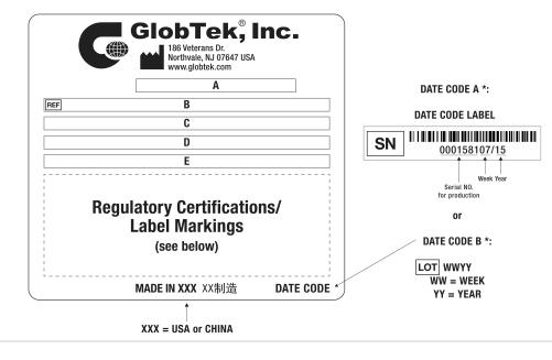
A=ICT / ITE / Medical Power Supply/Class 2/Household Power Supply B=P/N: (料号) WR9QA3000USBCRCIMR6W C=Model (型号) GTM96180-1507-2.0 D=Input (输入)100-240V~, 50-60 Hz, 0.6 A E=Output (输出)5.0 V ---- 3.0 A, 15.00W
