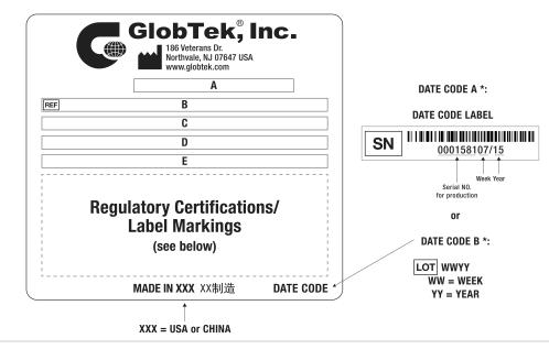
A=ICT / ITE / Medical Power Supply/Class 2/Household Power Supply B=P/N: (料号) WR9QA3000USBC25MNA-CIMR6B C=Model (型号) GTM96180-1507-2.0 D=Input (输入)100-240V~, 50-60 Hz, 0.6 A E=Output (输出)5.0 V ---- 3.0 A, 15.00W
